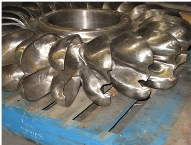
FIGURE 82: Damaged Pelton turbine blades 100
