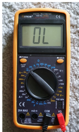
FIGURE 116: Continuity testing on multi-meter 134
