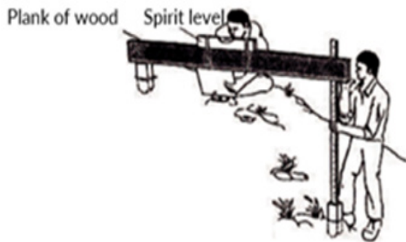
FIGURE 98: Spirit Level and Plank Method 116
