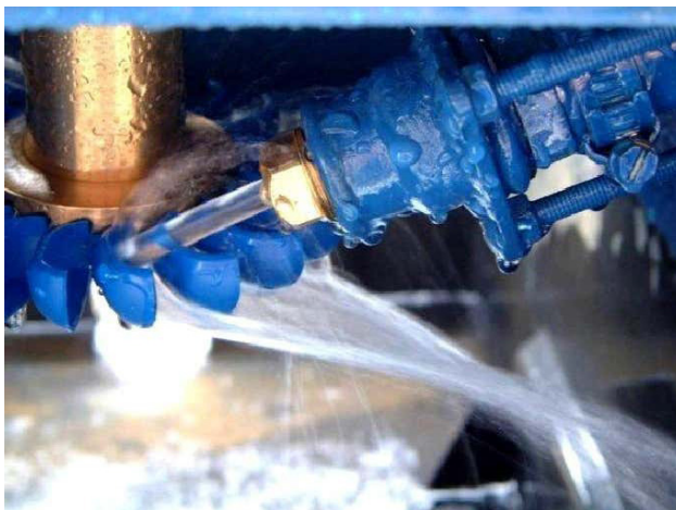
FIGURE 12: Water hits the buckets at an angle in Turgo turbines 12
