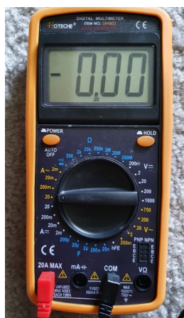
FIGURE 120: AC current measurement on multi-meter 138
