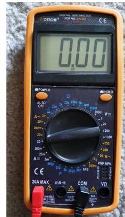
FIGURE 118: DC current measurement on multi-meter 136
