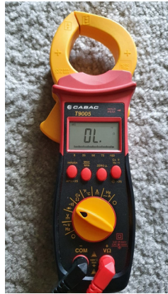
FIGURE 106: Continuity testing on clamp-meter 124
