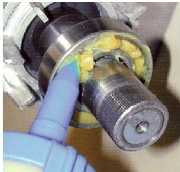
FIGURE 79: Greasing a bearing on shaft 97
