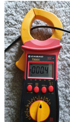
FIGURE 108: DC current measurement on clamp-meter 126
