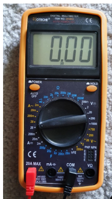
FIGURE 68: DC current measurement on multi-meter 71
