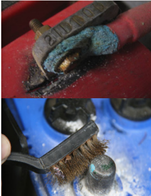
FIGURE 63: Cleaning Terminal Corrosion 66
