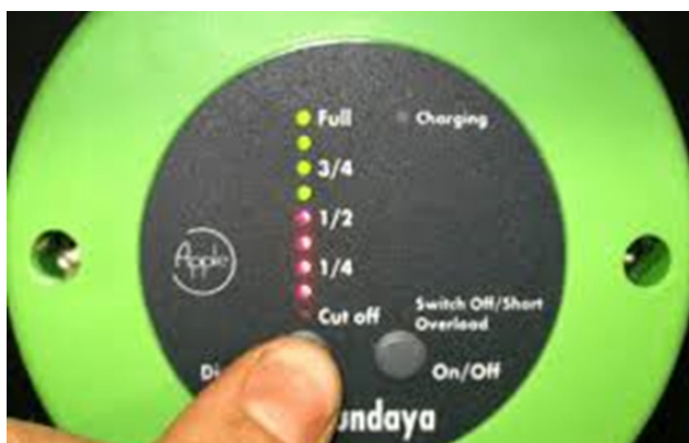
FIGURE 61: LED lights indicate the battery charge level 64
