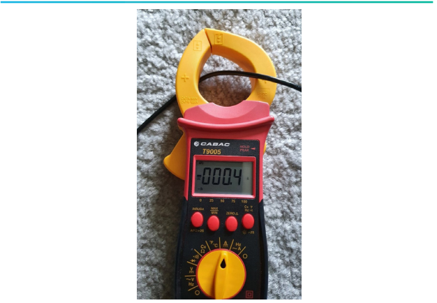
FIGURE 96: DC current measurement on clamp-meter 92
