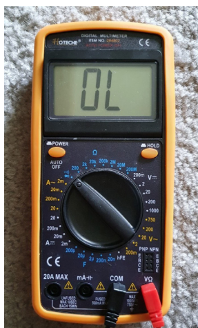
FIGURE 104: Continuity testing on multi-meter 100
