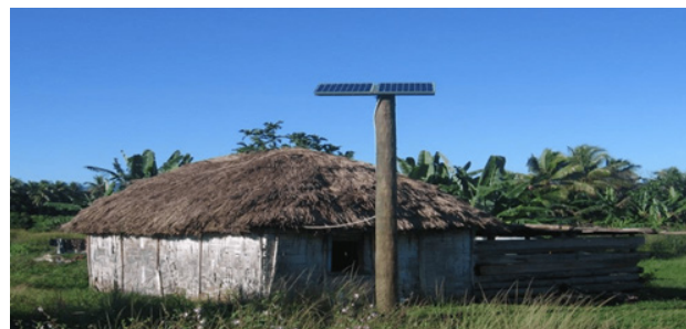
FIGURE 55: Pole mounted solar is better option due to unsuitable roof structures 52
