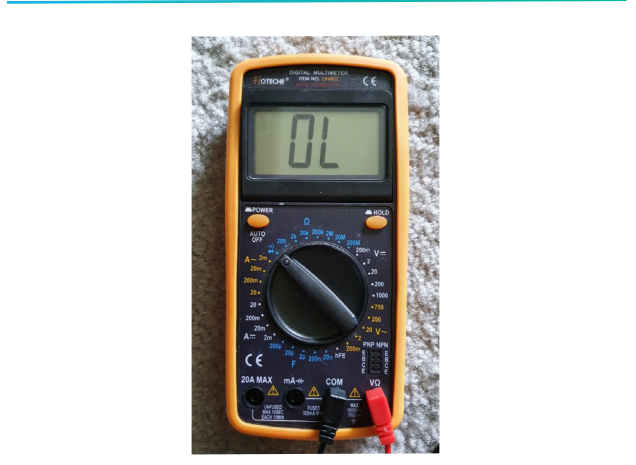
FIGURE 62: Continuity testing on multi-meter 70
