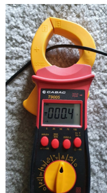
FIGURE 54: DC current measurement on clamp-meter 62
