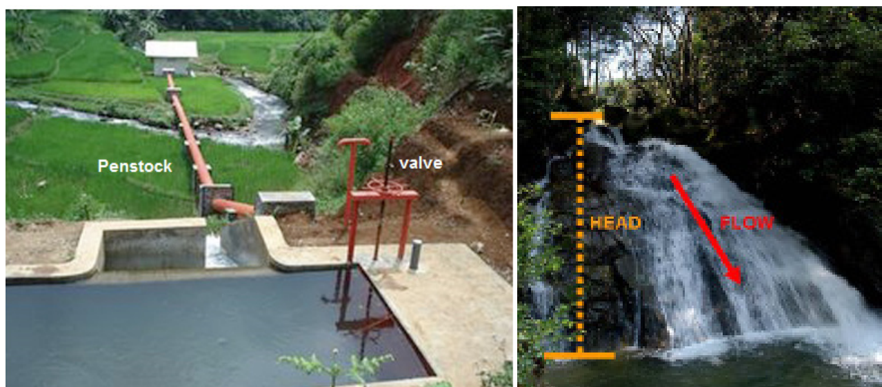
FIGURE 6: Schematic and pictures of a typical Pico-Hydro system 6
