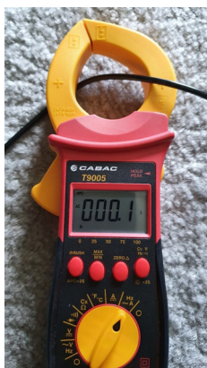
FIGURE 56: AC Current measurement on clamp-meter 64
