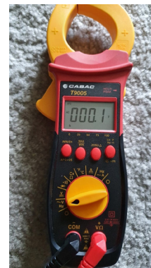
FIGURE 50 : AC Voltage measurement on clamp-meter 58
