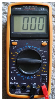
FIGURE 58: DC Voltage measurement on multi-meter 66
