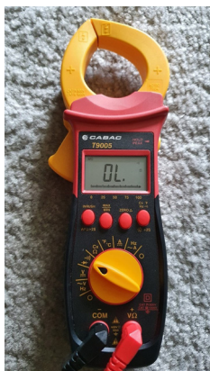
FIGURE 52: Continuity testing on clamp-meter 60
