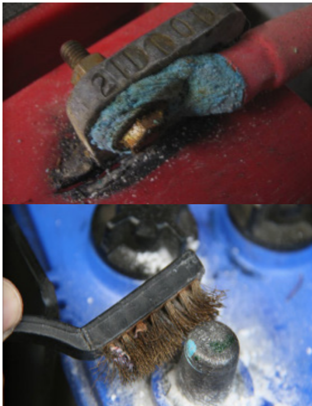
FIGURE 63: Cleaning Terminal Corrosion 64
