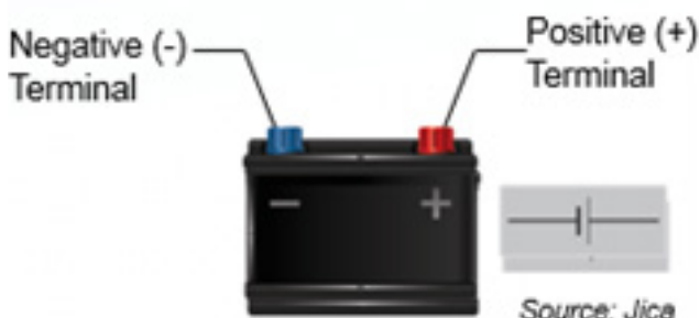
FIGURE 12: Polarity of Battery 12
