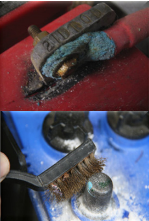
FIGURE 55: Cleaning Terminal Corrosion 55
