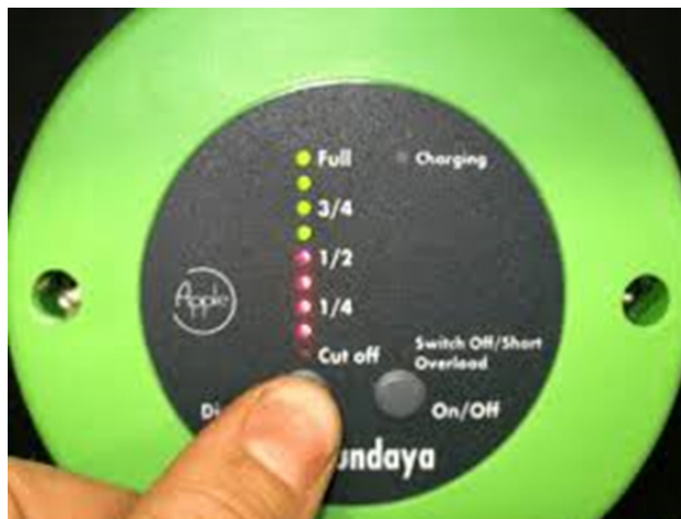
FIGURE 53: LED lights indicate the battery charge level 53
