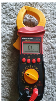
FIGURE 61: Continuity testing on clamp-meter 61
