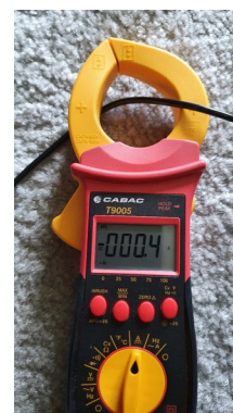
FIGURE 63: DC current measurement on clamp-meter 63
