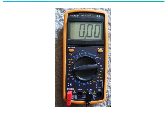
FIGURE 73: DC current measurement on multi-meter 74
