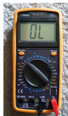
FIGURE 71: Continuity testing on multi-meter 71
