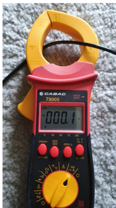
FIGURE 65: AC Current measurement on clamp-meter 65
