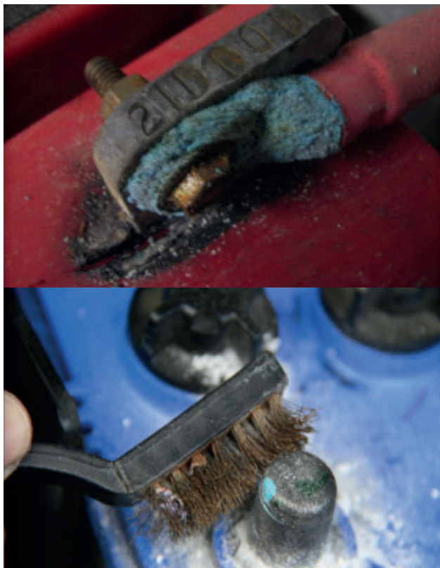
FIGURE 63: Cleaning Terminal Corrosive 66
