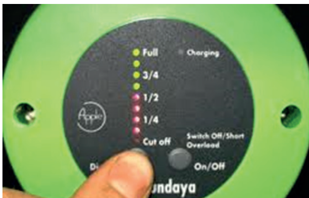
FIGURE 61: Led lights indicate the battery charge level 64
