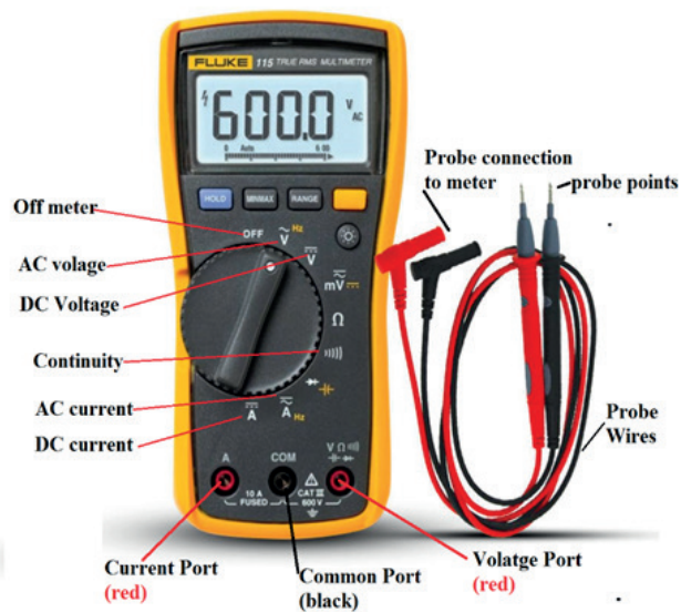
FIGURE 64: Parts of a multi meter 67
