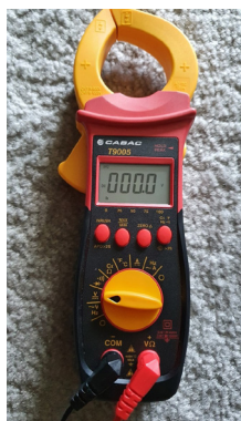
FIGURE 48: DC Voltage measurement on clamp-meter 56
