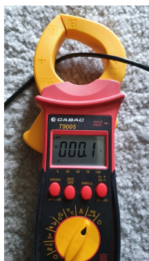
FIGURE 56: AC Current measurement on clamp-meter 64
