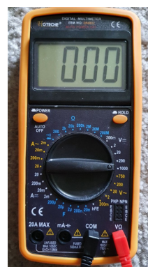
FIGURE 58: DC Voltage measurement on multi-meter 66
