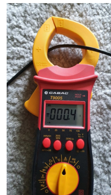
FIGURE 54: DC current measurement on clamp meter 62
