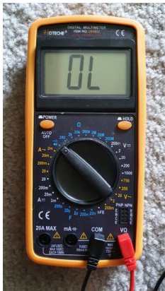
FIGURE 62: Continuity testing on multi-meter 70
