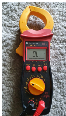
FIGURE 52: Continuity testing on clamp-meter 60
