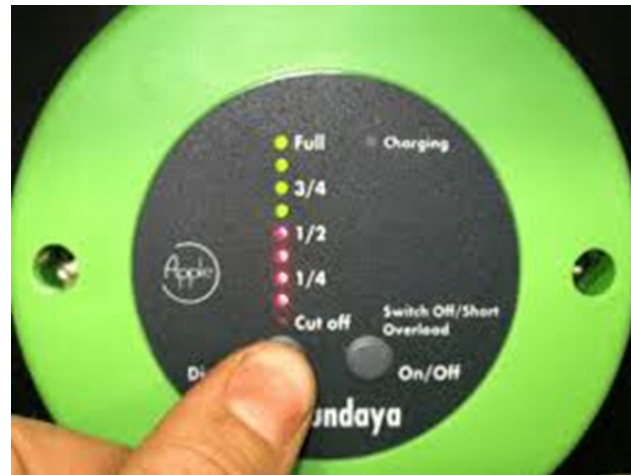
FIGURE 44: LED lights indicate the battery charge level 54
