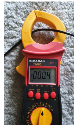
FIGURE 108: DC current measurement on clamp-meter 126
