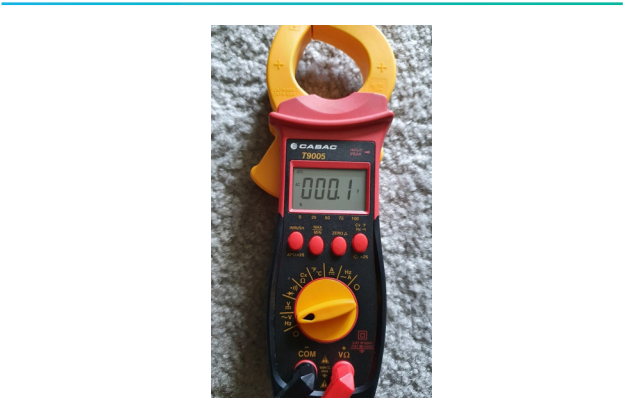
FIGURE 104: AC Voltage measurement on clamp-meter 122
