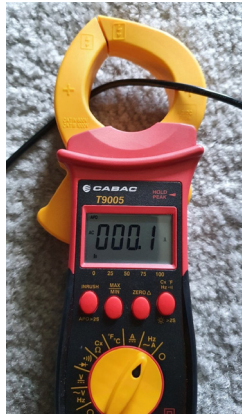
FIGURE 110: AC Current measurement on clamp-meter 128
