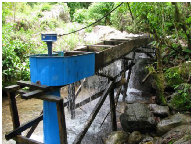
FIGURE 63: A Pico hydro turbine mounted on timber frames 82
