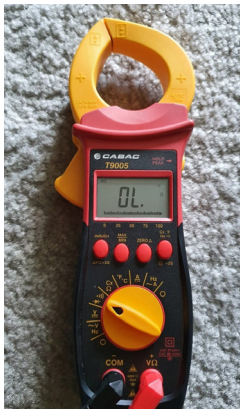
FIGURE 106: Continuity testing on clamp-meter 124
